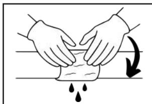
6. Dip gloves in water and smoothen pipe tape with hands in the direction of wrap until it sets
