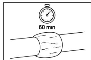
7. The pipe tape hardens after 10 min and fully cured after 60 min. (at 20 °C)
