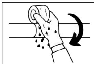
5. Wrap pipe tape firmly around pipe (min. 9 wraps with 50% overlap)
