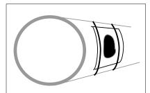
3. Cut a suitable piece of the metal mesh and fix it to the repair area using steel band or steel wires.
