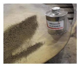
6. Due to the extent of cavitation and damage to the propeller blades, the surface is already rough and suitable for applying Wencon Ceramic Cream.
