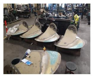
9. 2<sup>nd</sup> and final layer of Wencon Ceramic Cream applied in layer thick enough to ensure level above to original surface has been obtained.
