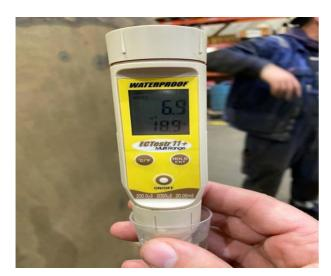
4. Measured salt content of the liquid after injection in patch x 5 times - value measured 6.9 us / cm
