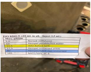
5. The final value: 2.5-6.9 = 4.4 us/cm. According to the most common standards as seen on picture on the left, it will meet even the toughest standards.
