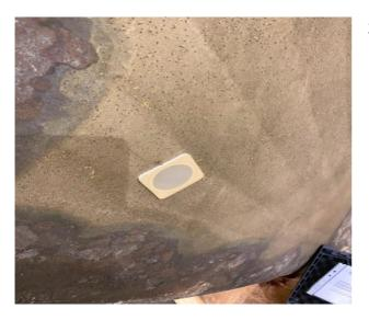
2. After disassembling the Propeller Blades, the surface is prepared using UHP Water Jetting to remove all salt and uncleanness's out if the metal surface.
