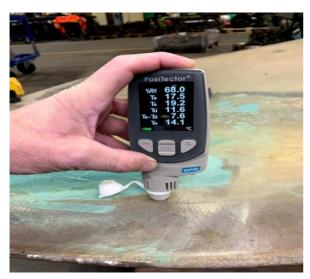
10. Throughout the complete application process, distance to the dew point is kept above 3°C to ensure a dry surface to be applied to.
