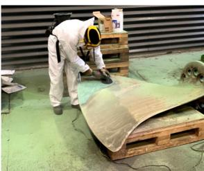
11. Subsequent to final curing has occurred, the original shape and size of the Propeller Blades is recovered by using grinding tools and ordinary polish tools as normally used to polish the Propeller Blades.
