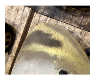
7. Cavitation damage on the Propeller Blade.
