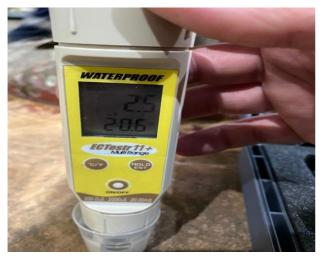
3. Measured salt content of the liquid before injection of the liquid into the patch – value 2.5 us/cm
