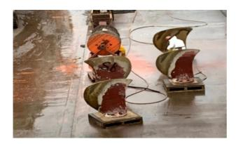
1. After disassembling the Propeller Blades, the surface is prepared using UHP Water Jetting to remove all salt and uncleanness's out if the metal surface.
