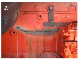
3. Holes were drilled in the outer end, directly in the crack, with a interval of 5 cm to prevent elongating
