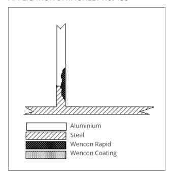
Drawing shows corrosion in the area, where steel and aluminum meet. The corrosion is of bimetallic nature, and is very simple to repair (avoid) with Wencon.
