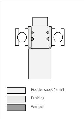
When removing a bushing, from a rudder stock or any other shaft, there might be created scores. In most cases this damage can be repaired with Wencon.
