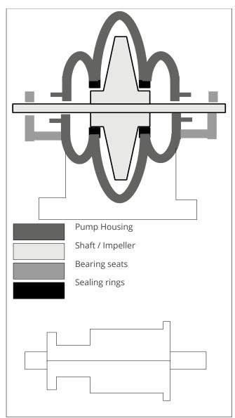
Corroded sealing seats and stuffing box housings are normally repaired by welding and line boring, but it is a long and costly process.
