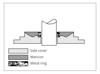
When a pump housing is suffering from deterioration, caused by a high degree of wear, from pumping sand and stones i.e. additional protection is recommended. For this repair we reinforce the area using a steel ring and Wencon Aggregate to increase the wear resistance.
