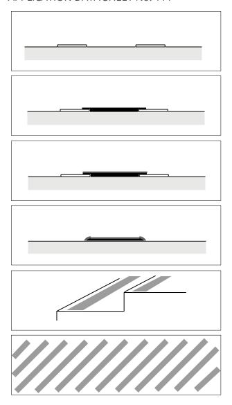
Wencon Coating and Aggregate are used to ensure non-slip surfaces in different situations. Most common applications are non-slip surfacing of floors, steps, stairs, passages etc. It is of equal interest to name conveyor belt drive rollers, forks on fork-lift trucks, rear loading ramps on lorries, and steps on cars or other transport machines. The system is very simple to use. Apply Wencon Coating to the surface to be treated, and sprinkle Wencon Aggregate on top.
