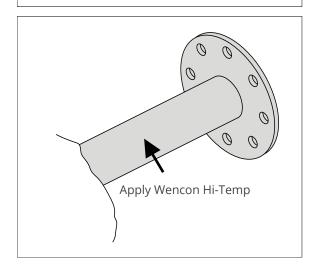
Hot-water, hot-oil or steam pipes will often be exposed to corrosion on the outer side, due to moisture or water in the insulation. Wencon can eliminate this breakdown with a coat of Wencon Hi-Temp.
