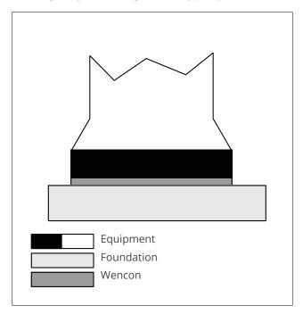
Chocking, grouting or casting of resins for the purpose of creating a strong connection between foundation and equipment, has become more common in the marine industry.
