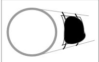
4. Apply second layer of the compound and leave it for initial curing for 3-4 hours, depending on temperature and humidity.
