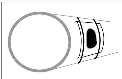
3. Cut a suitable piece of the metal mesh and fix it to the repair area using steel band or steel wires.
